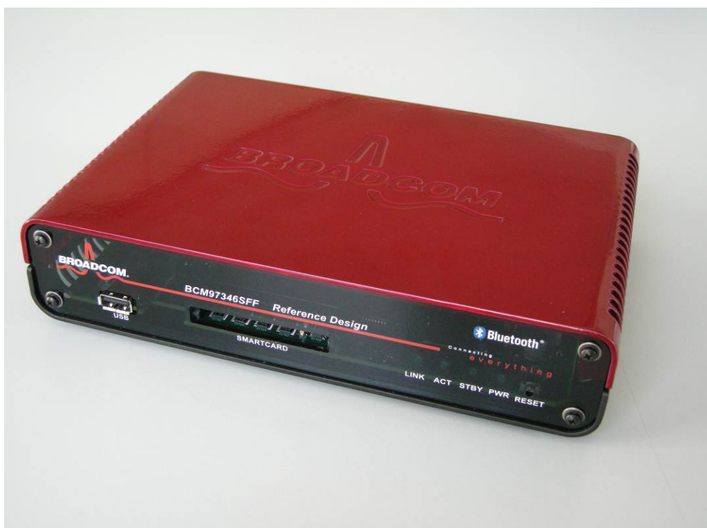
Figure 16: Broadcom reference set-top-box for chip-set BCM7346
