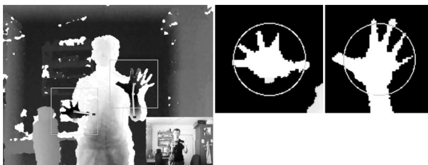
Figure 16: Detected hands are segmented from the main picture in order to minimize image processing complexity
