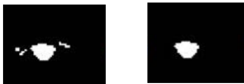
Figure 23: a) Image after CDF b) Image a) after erosion morf. oper.
