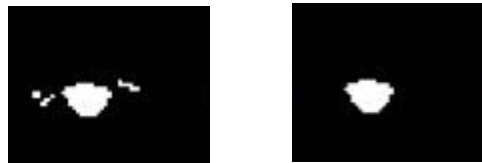
Figure 8: a) Image after CDF b) Image a) after erosion morf. oper.
