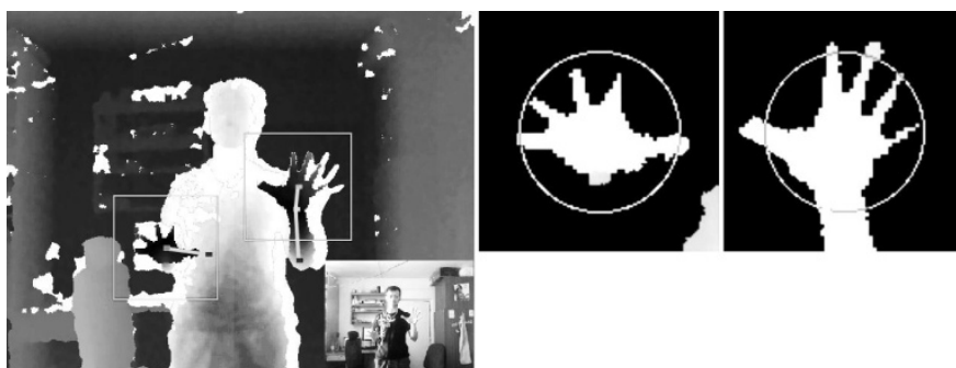
Figure 3: Detected hands are segmented from the main picture in order to minimize image processing complexity
